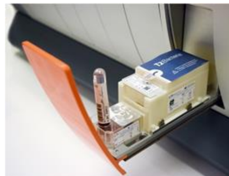
The T2Bacteria Panel is placed into the T2Dx Instrument to identify sepsis-causing bacteria directly from whole blood
