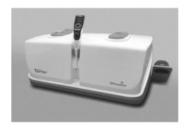
We have also applied T2MR to develop the T2Plex, which is a compact, fully integrated instrument capable of rapidly providing comprehensive hemostasis measurements, including platelet function, clotting time and clot degradation, also known as fibrinolysis.
